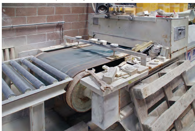
The output conveyor of the Gisbert production line
